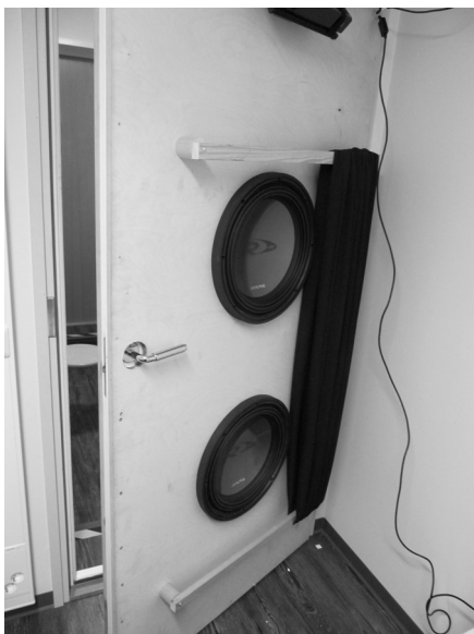
FIG. 1. Loudspeaker drivers were attached to the reinforced door of the chamber and hidden behind a curtain during tests.
